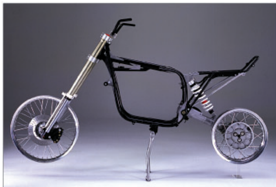
At the stripped skeleton you see the reinforcements of the frame.
