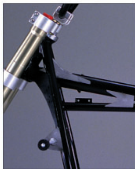
Reinforced steering head area, for better driveability and higher loads.
