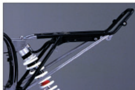
Reinforced rear section and mounting points of the shock absorber are designed for highest stresses.
